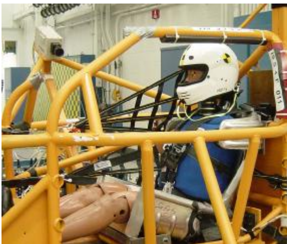
Rally Net Test w/ LFT Technologies R3 – Note Location of upper strap through cg of the head.
