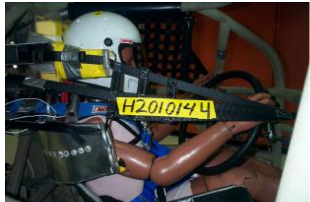
Net Sled Test 2001 – 50 G impact
