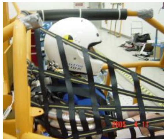
Rally Net Test w/ LFT Technologies R3 – Note Location of upper strap through cg of the head.
