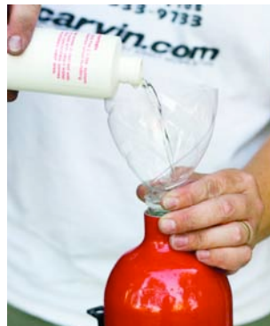
(ABOVE) We installed the actuator using a reinforced plastic cover where the radio once resided. (RIGHT) Be careful when handling the AFFF, as the chemical can be harmful to the eyes before it's mixed with water. (BELOW) Installed, the fire system doesn't take up much space. Be sure to remember to remove the safety pins before racing.
