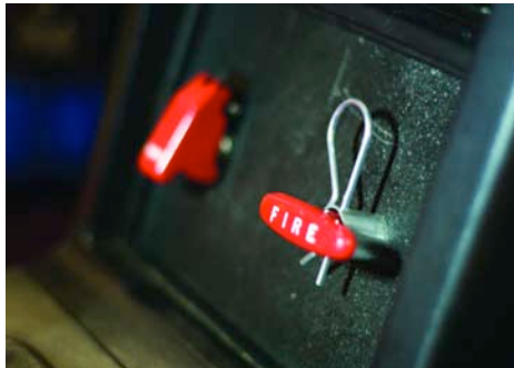
(ABOVE) We installed the actuator using a reinforced plastic cover where the radio once resided. (RIGHT) Be careful when handling the AFFF, as the chemical can be harmful to the eyes before it's mixed with water. (BELOW) Installed, the fire system doesn't take up much space. Be sure to remember to remove the safety pins before racing.
