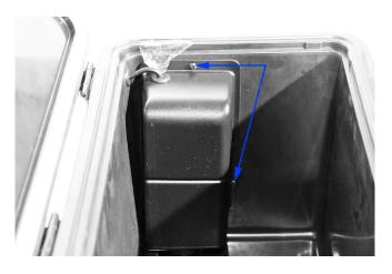
Remove 2 screws that secure the pump shroud
